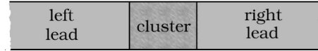
FIG. 11. Geometry used for the calculation of the conductance. The interacting region (cluster) is connected by ideal contacts to semi-infinite ideal leads.
