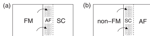
FIG. 1. Schematic representation of the systems studied here. (a) is a heterostructure involving a ferromagnetic (FM) half-metal system, such as LCMO, and a superconductor (SC), such as YBCO. In this case, an antiferromagnetic (AF) insulating state is induced at the interface. (b) is a heterostructure involving a non-FM manganite and an undoped AF cuprate. Here, the transfer of charge may lead to a superconducting state at the interface. Arrows indicate the direction of flow of electrons, which are accumulated in the gray region.
