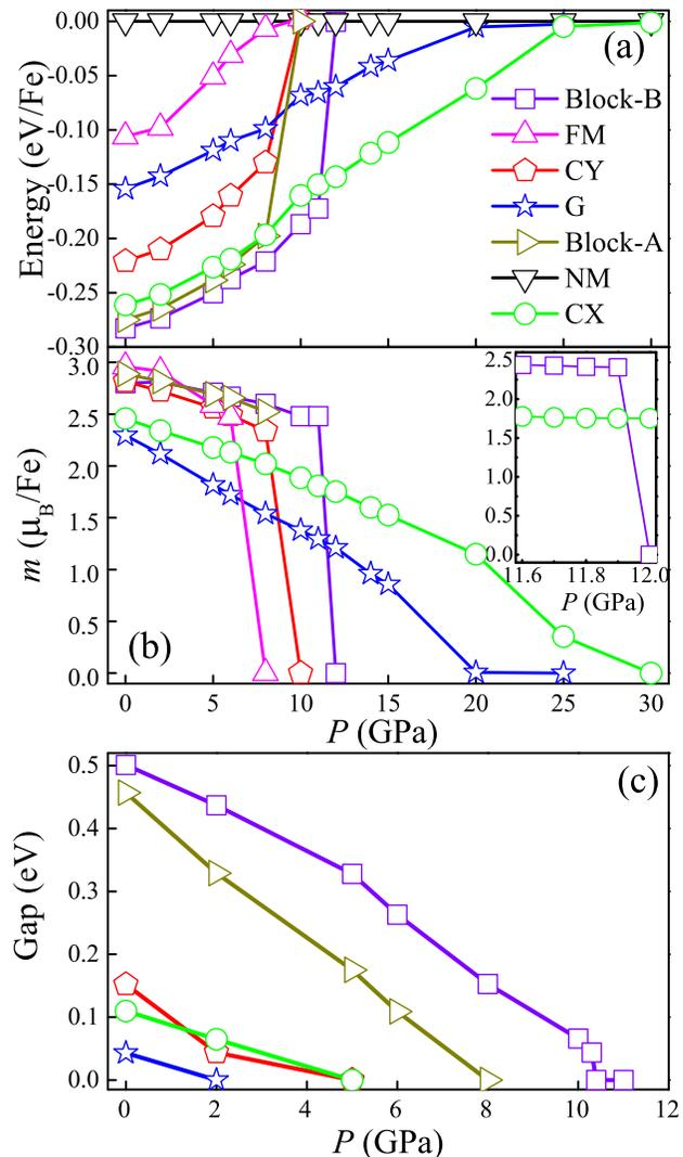
FIG. 2. Evolution of the magnetic and electronic structures of  $\text{BaFe}_2\text{Se}_3$  as a function of pressure. (a) Energies (per Fe) of the various magnetic orders indicated. (b) Local magnetic moments of Fe, integrated within the default Wigner-Seitz sphere as specified by VASP. *Inset*: an amplified view near the transition. (c) Band gaps for the many states analyzed.
