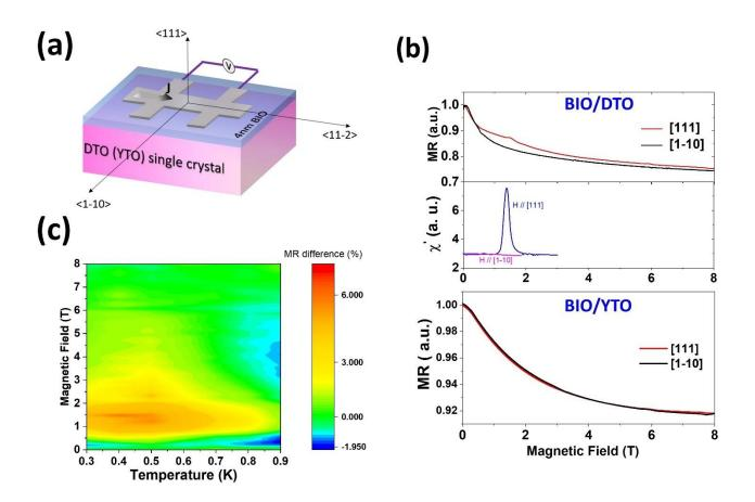
Figure 2 (a) schematic diagram of the measurement with BIO/DTO(YTO) heterostructure. (b) (top) measured MR for the BIO/DTO heterostructure at 0.3 K with H // [111] (red) and H // [1-10] (black), with AC susceptibility measured at the same temperature with H // [111] (blue) and H // [1-10] (pink). (bottom) MR for the BIO/YTO heterostructure shows no similar anomaly. (c) color plot of the MR difference with H//[111] and H[1-10], measured between 0.3 K and 0.9 K.
