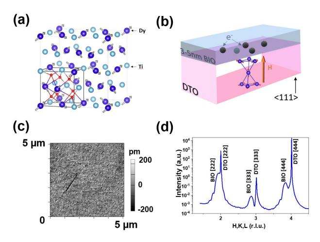
Figure 1 (a) crystal structure of  $Dy_2Ti_2O_7$ , the Dy and Ti atoms each form corner-sharing tetrahedra. Oxygen atoms outside the solid cube are not shown for clarity purpose. The spins on the Dy sites show the '2-in-2-out' configuration. (b) designed heterostructure with a 3-5nm BIO thin film deposed on the DTO single crystal. (c) The AFM image of the DTO substrate surface. (d) Synchrotron x-ray diffraction covering the DTO [222] to [444] region.
