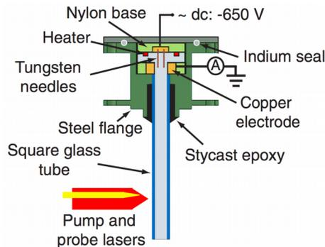
FIG. 1 Schematic diagram of the counterflow channel used in the molecule tagging experiment.
