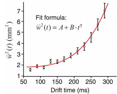
FIG. 5 The square of the width of a molecule line  $\bar{w}^2(t)$  as a function of drift time  $t$  at a heat flux of  $277 \text{ mW/cm}^2$
