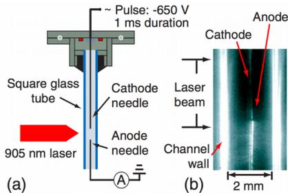
FIG. 6 (a) Schematic diagram of the counterflow channel used in the cluster tracking experiment. (b) An image of the square glass tube. A pulsed laser at 905 nm illuminates the needle apexes at about 2 cm from the open end of the channel.
