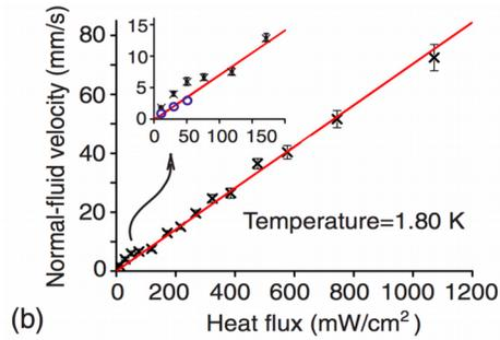
FIG. 8 The obtained normal-fluid velocity as a function of heat flux at 1.80 K. The black crosses are the data. The red line shows the calculated normal-fluid velocity based on Eq. (1) in the text. The blue circles in the inset for the small heat flux regime show the corresponding measured normal-fluid velocity divided by a factor of 2.
