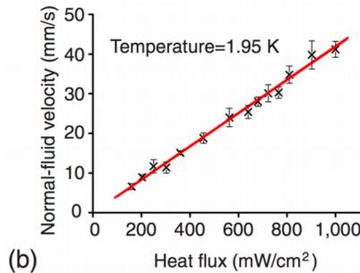
FIG. 4 The obtained normal-fluid velocity as a function of heat flux at 1.95 K
