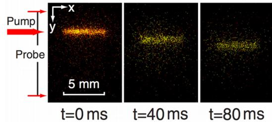
FIG. 2 Typical fluorescent images of a line of helium molecules taken at a heat flux of  $640 \text{ mW/cm}^2$  and pump-probe delays of 0, 40, and 80 ms, respectively.
