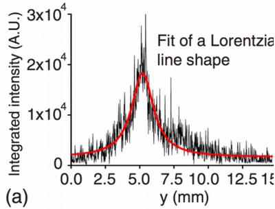
FIG. 3 A typical integrated cross-section profile of a molecule line in arbitrary units. The red line is a Lorentzian fit to the data.
