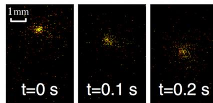
FIG. 7 Typical fluorescent images of a cluster of helium molecules taken at 0, 0.1, and 0.2 s after the cluster was created. The heat flux is  $119 \text{ mW/cm}^2$ . The temperature is 1.80 K. The exposure time for each image is 20 ms.
