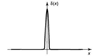
$$\delta(x) \equiv \left\{ \begin{array}{ll} 0, & \text{if } x \neq 0 \\ \infty, & \text{if } x = 0 \end{array} \right\}, \quad \text{with } \int_{-\infty}^{+\infty} \delta(x) \, dx = 1$$
