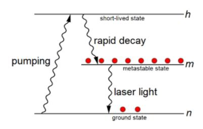
This is the basis of Light Amplification by Stimulated Emission of Radiation (LASER).
