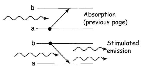
Amplification can occur. Almost instantly a huge number of photons in phase can be produced:
