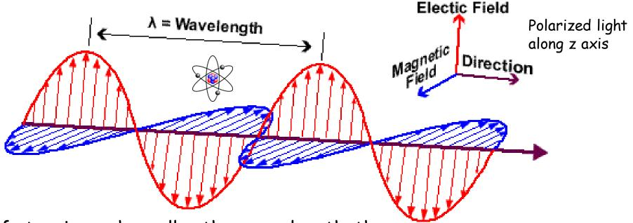
If atom is much smaller than wavelength, then the electric field is ~ uniform inside atom
