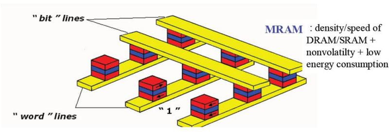
Figure 5: A schematic diagram of mram
