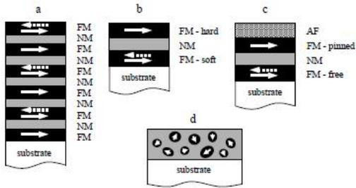
Figure 3: These are four examples of systems that show GMR. A) is layered magnetic, non-magnetic layers B) and C) are both examples of spin valves D) is a granular sample.
