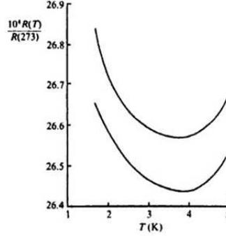
Figure 5: The minimum in the electrical resistivity of Au. (de Haas, de Boer and Van den Berg, 1934)
