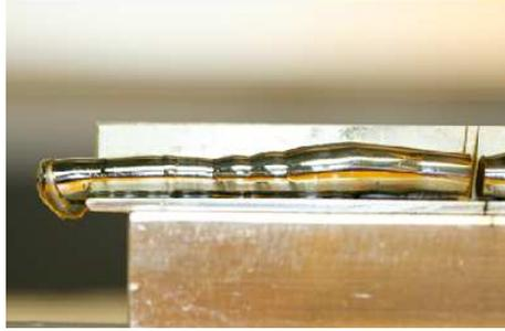
Figure 1: 20 grams of  $UPt_3$  single crystals grown at Northwestern University
