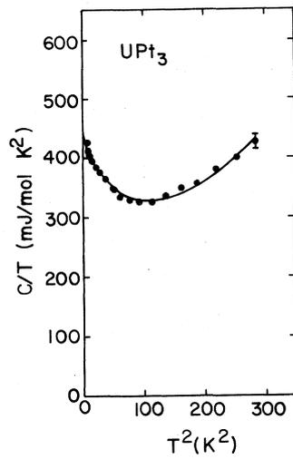
Figure 3: Specific heat in the normal state of flux-grown single crystals of  $UPt_3$  [3]. The line through the data is a least-squares computer fit of the data to  $C = \gamma T + AT^3 + \delta T^3 \ln T$ .
