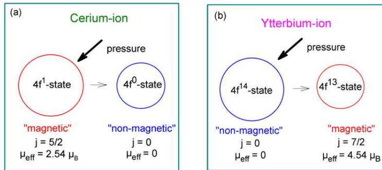
Figure 9: schematic explanation for the function of pressure application.
