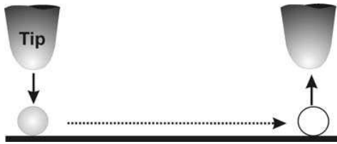
FIG. 13: STM performing lateral mode manipulation [12]
