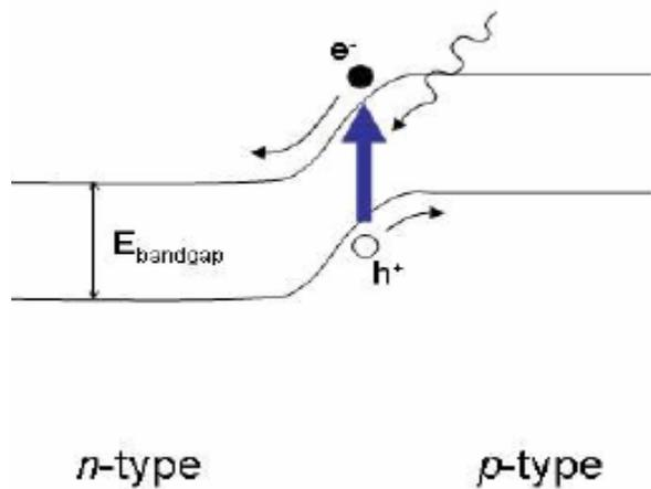
In p-n junction, due to the inside electric field, the electron and hole will move in opposite directions and finally be separated. This is the way silicon semiconductor generate current under sun light.
