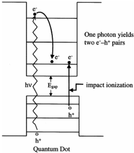
Another very important feature is that, technically, Quantum dot's band gap is easily to be set. It means we can choose the light with which kind of wavelength we want to choose. Different kinds of Quantum dots cell span almost all solar energy spectrum.
