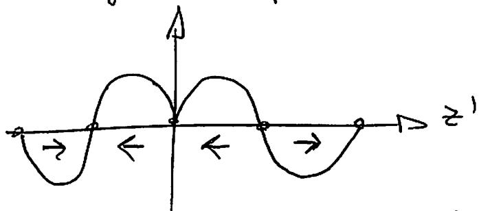
indicates that this is a combination of "4 dipoles" as indicated by arrows. The total dipole cancels and only the quadrupolar component survives.
