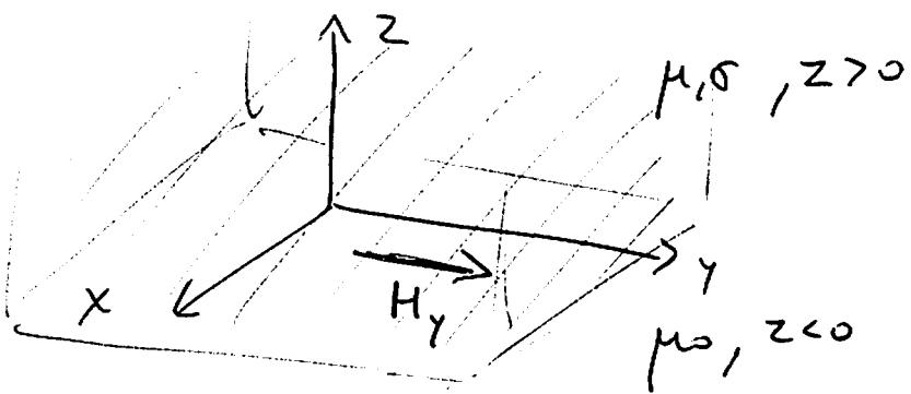
$$H_y = H_0 \sin(\omega t) \text{ at } z=0-\epsilon (\text{or } 0^-)$$
