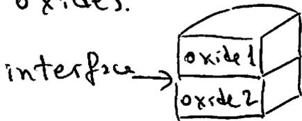
Modern "growth" techniques, called "pulsed laser deposition" and "molecular beam epitaxy" allow the growth of layers of oxides one over the other with atomic accuracy.
